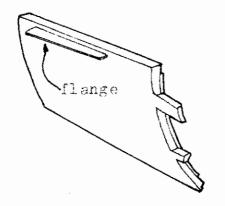
SPEED BRAKE DOORS: note that the doors have a thin flange attached to them at the upper edge of the door. The flange tapers from rear to front(i.e., narrower at the forward end than the rear end...but you already figured that out...)
