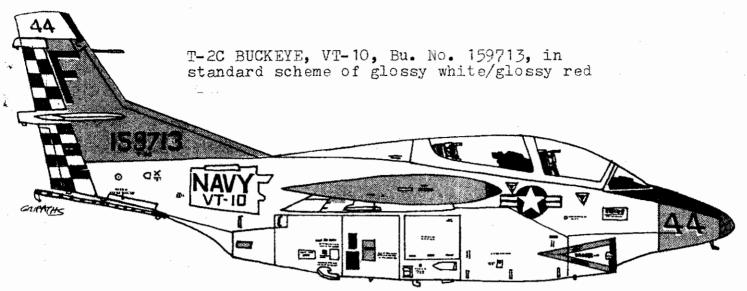
Note that '44' on tail and nose lean backwards; '44' on nose shadow-edged in white. 'F' on tail leans rearward also and is shadow-edged in white. Rudders in checkerboard of blk. & whte. Intake chevron red w/ white lettering; intake lip in flt. blk. Anti-glare panel in bkack and has the tiniest sheen to it; radome in a faded brownish-grey color(very flat). '44'on flaps and under wing ahead of port gear door. A/c profusely stencilled.
